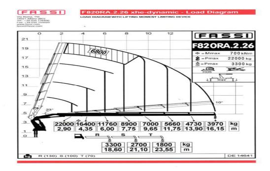
Crane Capabilities with fly jib (standard 6 extensions with 4 extension fly jib)
